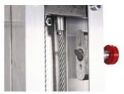
Safety pins: Allow selecting different heights and spreading the load to all bars equally.
