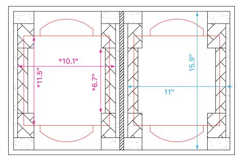
\*Foam inserts can be removed or modified to extact area of the wood edges.
